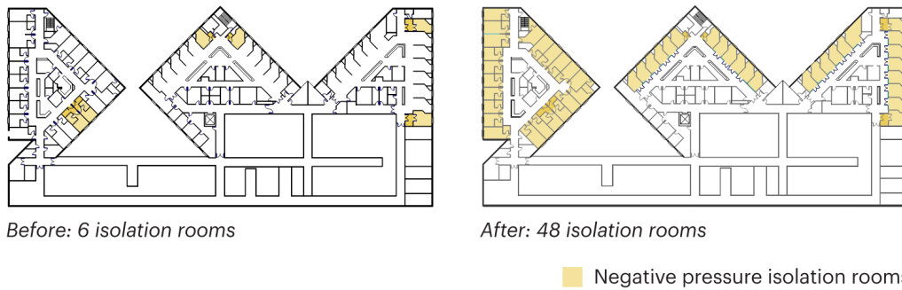
Figure 8: Negative pressure isolation rooms on 6th floor of Guggenheim Pavilion, image copyright MASS Design Group.
