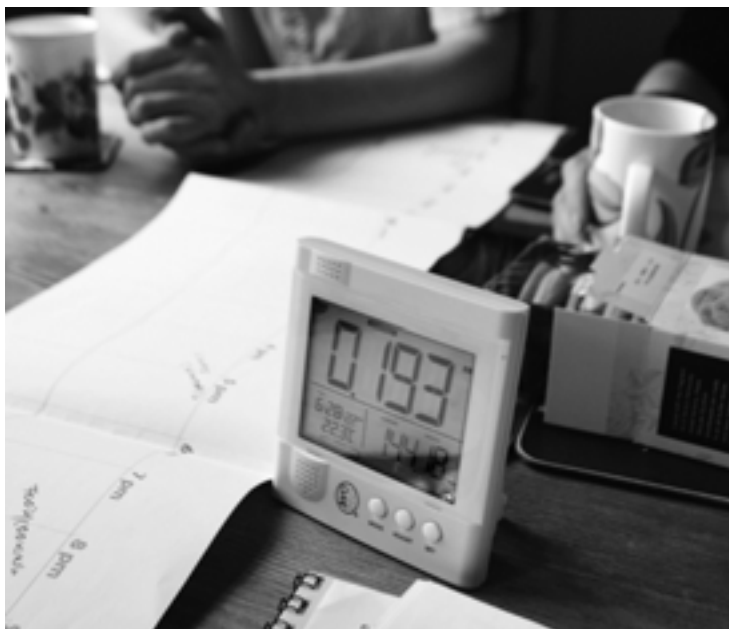
FIGURE 1. An example of an OWL electricity real-time display in use by two of our participants, Jerry and Amy. The device shows real-time and cumulative electricity use (in kW and kWh), time, air temperature and can also show costs and carbon footprint in kg CO 2 equivalent.
