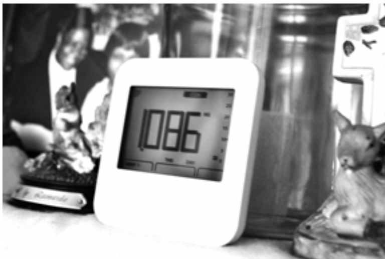
FIGURE 6. Edith uses her OWL electricity display in the ‘kg CO 2 equivalent’ mode, showing her estimated daily carbon footprint from electricity use.
