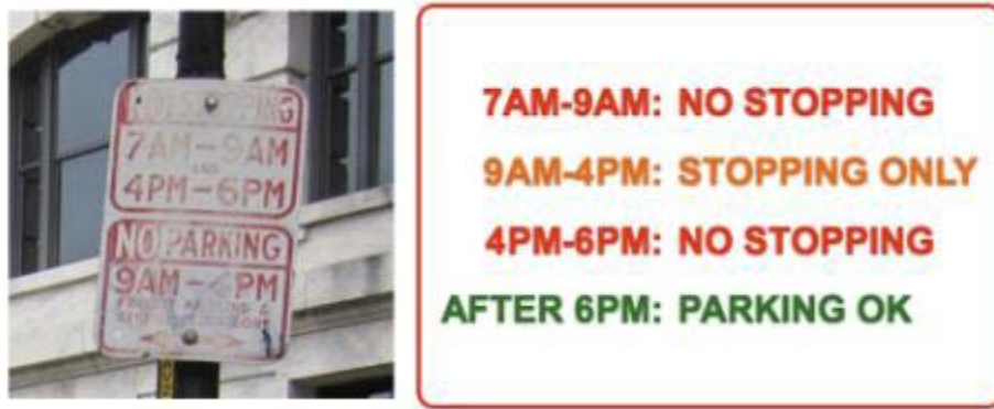
FIGURE 10. A proposed redesign of the sign on the left to help drivers quickly determine what they can do right now as they drive by.
