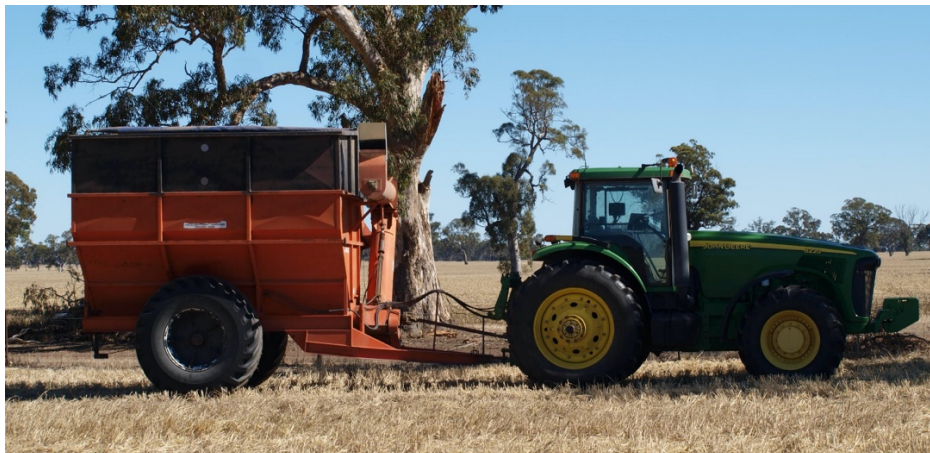
Figure 6. The black top third of the chaser bin shows where it has been extended by the owner. (Photograph taken by the first author)
