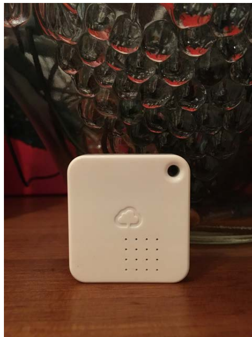
Figure 2. Ambient temperature sensors throughout the flat – on radiators and placed on the walls on 1.2 meters height, for the most accurate results (product: Wireless Sensor Tags Canada).
