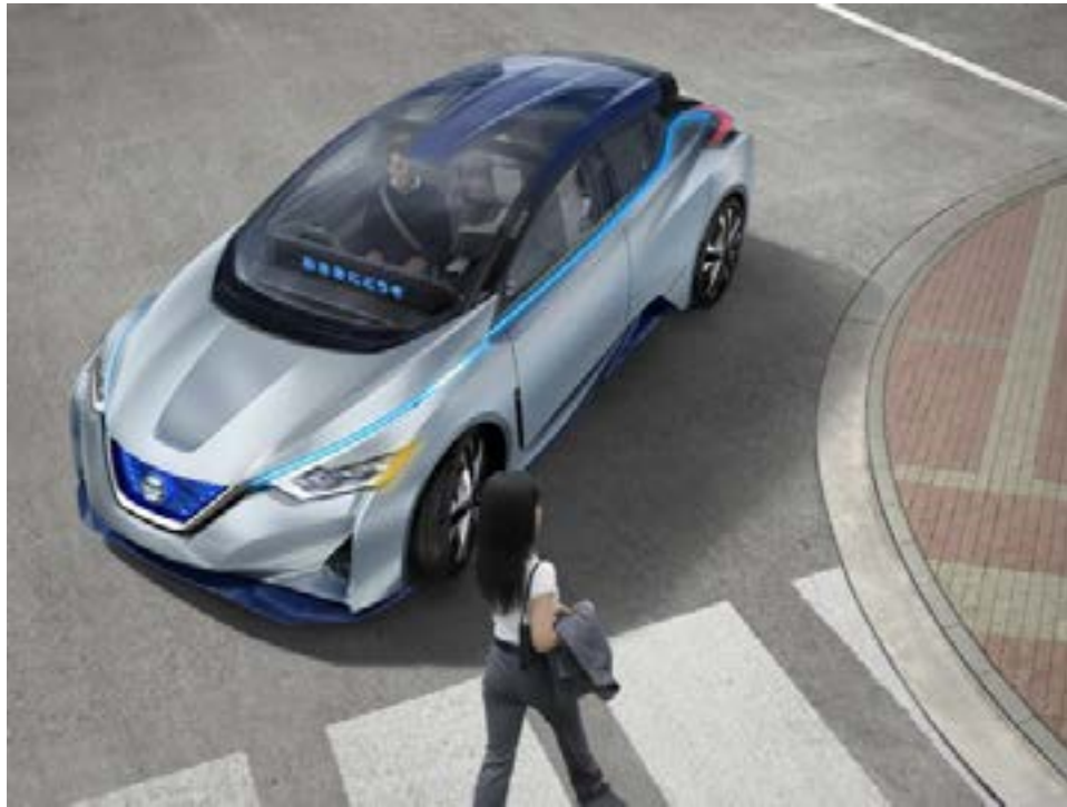
Picture 8. The Nissan IDS concept car with the intention indicator represented by the blue light strip running along the sides and front of the car, as well as a display in the window.
